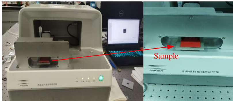
Fig. 6. THz-TDS testing device diagram and test sample
