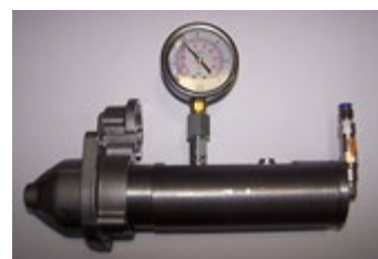
Fig. 2. Gas leakage testing station (casting leak testing)
