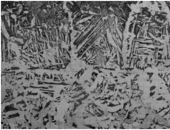
Fig. 4. Casting 1 connection zone, magnification x50
