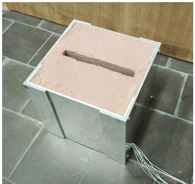
Fig. 1. Casting mould made from the tested molding sand reproducing the shape of a plate meeting the infinite plate condition
