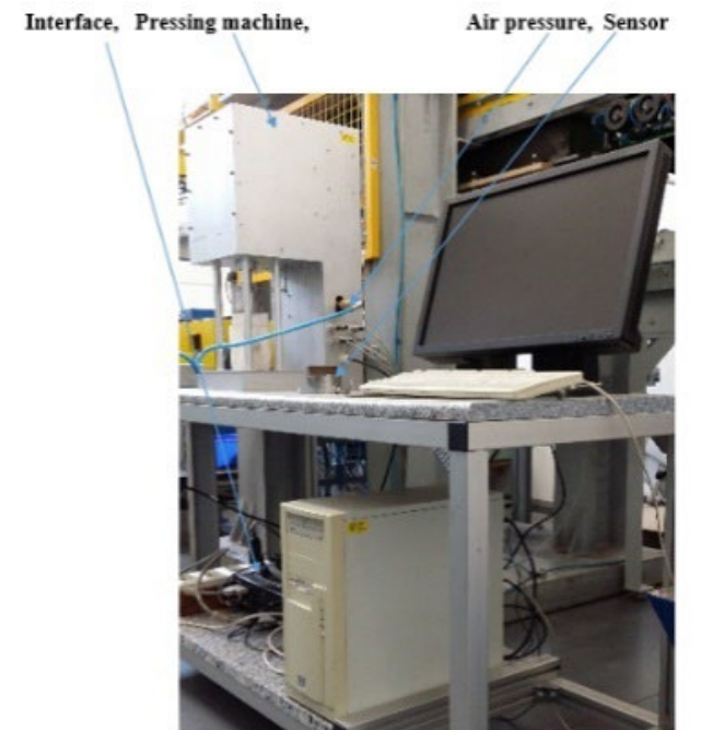
Fig. 1. An interface connects a computer, pressing machine and sensor
