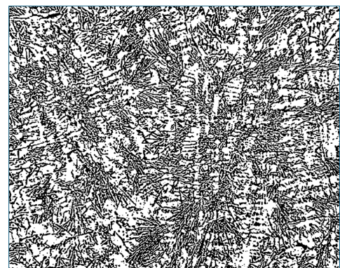
Fig. 5. Microstructure of the AlSi10Mg alloy cast by gravity casting into a mould made of shell mould material, mag. x200.
