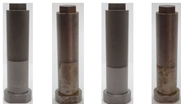
a) component 3D-3 before operational testing b) component 3D-3 after operational testing c) component 3D-4 before operational testing d) component 3D-4 after operational testing
