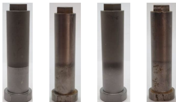
a) component C-3 before operational testing b) component C-3 after operational testing c) component C-4 before operational testing d) component C-4 after operational testing
