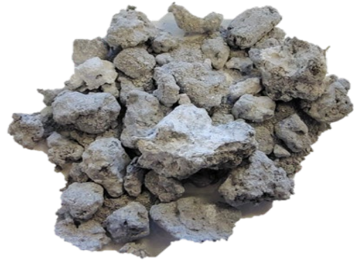
Fig. 2. Visual appearance of the post-refining dross before sample preparation
