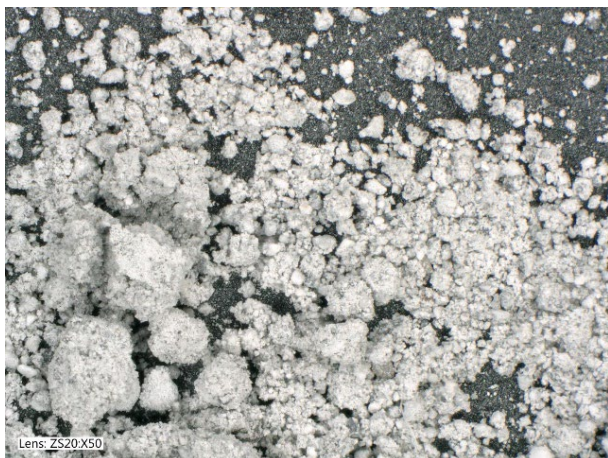
Fig. 4. Particle morphology of post-refining dross (50× magnification)
