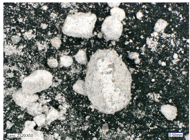
Fig. 3. Particle morphology of rotary furnace dross (50 \times magnification)
