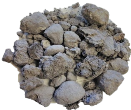
Fig. 1. Visual appearance of the rotary furnace dross before sample preparation
