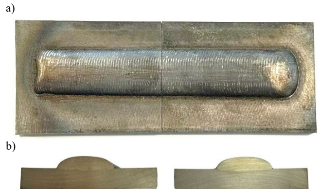
Fig. 3. View of the weld overlay deposited onto the cast iron substrate (a) and cross-section through the weld overlay sample (b)
