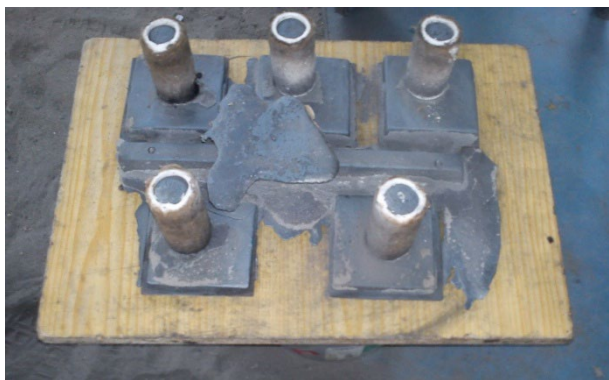
Fig. 5. Obtained castings: a) bimetal castings without preheaters, b) bimetal castings with preheaters (view from the preheater side)
