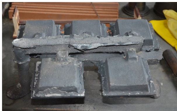
Fig. 5. Obtained castings: a) bimetal castings without preheaters, b) bimetal castings with preheaters (view from the preheater side)
