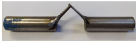
Fig. 2. The prepared shear-tensile test specimen
