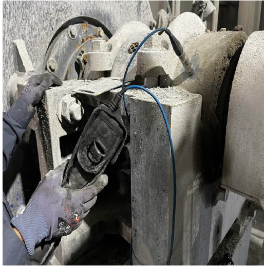
Fig. 15. Experimental setup for vibration data acquisition from the housing pump bearing
