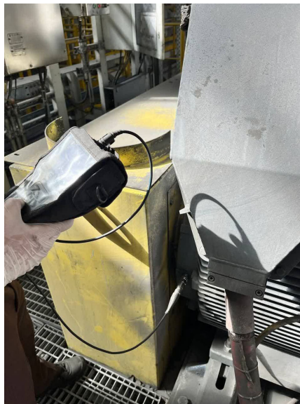
Fig. 12. Experimental setup for vibration data acquisition from the rougher bearing
