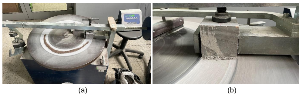
Fig. 4. Böhme abrasion test: (a) test stand, (b) rock sample during the test
