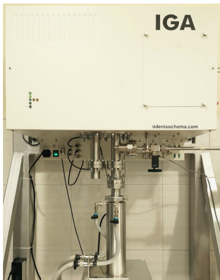
Fig. 6. IGA-001 measuring device
