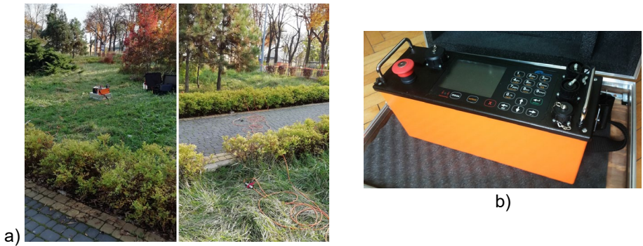
Fig. 5. The survey site view (a) and the ARES II unit used for measurements (b)
