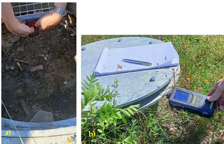
Fig. 13. Measurements: (a) backfill level; (b) gas concentration
