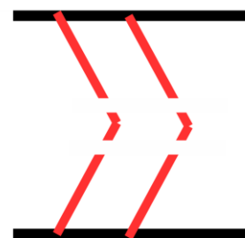
Fig. 34. Roughness elements in the form of discrete V-shaped ribs (drawn after [113]).
