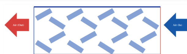
Fig. 59. Roughness element in the form of novel staggered cuboid baffles (drawn after [140]).
