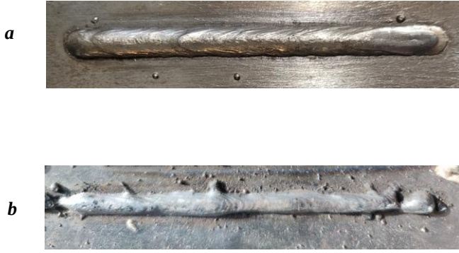
Fig.1. Weld images from the database, where: a) acceptable welds and b) unacceptable welds.
