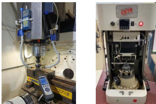
(a) The burnishing operation (b) Measuring coefficient of friction and wear depth Fig. 3. Experimental setting of the burnishing process
