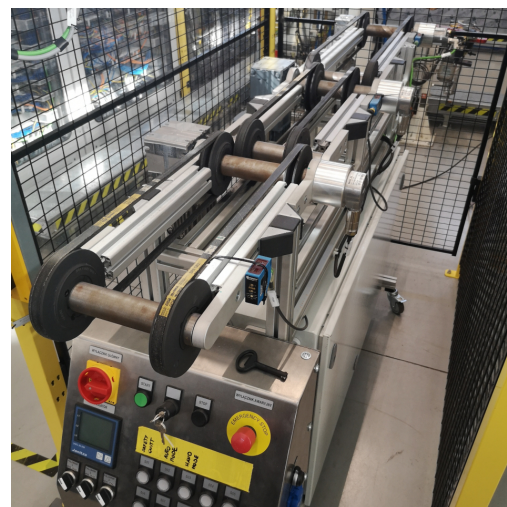
Fig. 1. Belt conveyor controlled by PLC Siemens S7-300
