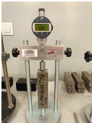
Fig. 4. Standard linear shrinkage test (LST): measuring setup (left); shrinkage evolution and comparison with model predictions (right)
