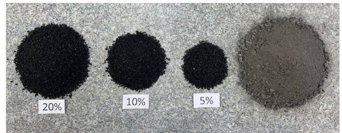
Fig. 1. Comparison of the colliery spoils sample with the applied crumb rubber additive
