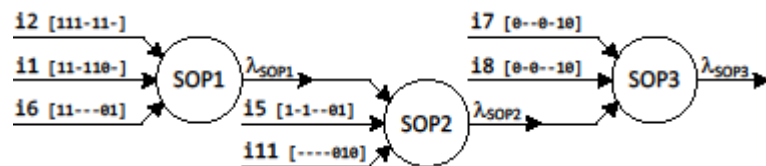
Fig.5. Technological representation of the analyzed function after creating three SOP blocks (SOP1, SOP2 and SOP3)
