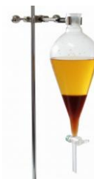
Fig. 1. Separation of reaction products into two distinct phases following transesterification and 8-hour settling period.
