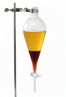
Fig. 1. Separation of reaction products into two distinct phases following transesterification and an 8-hour settling period
