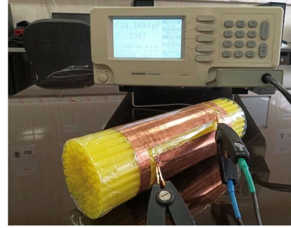
FIGURE 2. Measuring different volume fractions of the made experimental sensor.
