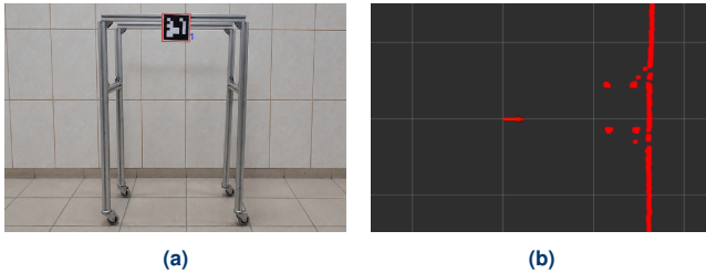
Fig. 9. Comparison of how the trolley placed near a wall is visible on camera and using LiDAR data. (a) Front view of the trolley using an RGB camera and featuring the detected and correctly recognized ArUco marker. (b) Top-down view of representation of the robots vicinity using LiDAR data, where the robots position is described using an arrow.
