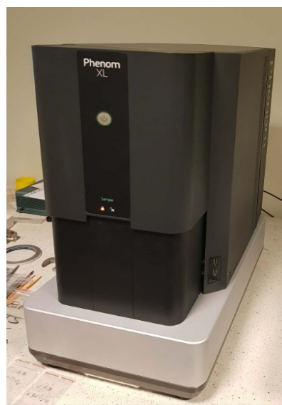
Figure A4. Thermo Scientific Phenom XL G3 Desktop SEM; accelerating voltage 5–20 kV; CeB 6 source; max. magnification 200000 \times .
