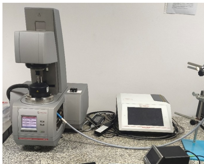
Figure A3. MCR302e rheometer equipped with an optical curing module; samples irradiated with 405 nm LEDs ( \approx 19.8 \text{ mW}\cdot\text{cm}^{-2} ) controlled by a DC2200 supply; temperature maintained at 25 °C.
