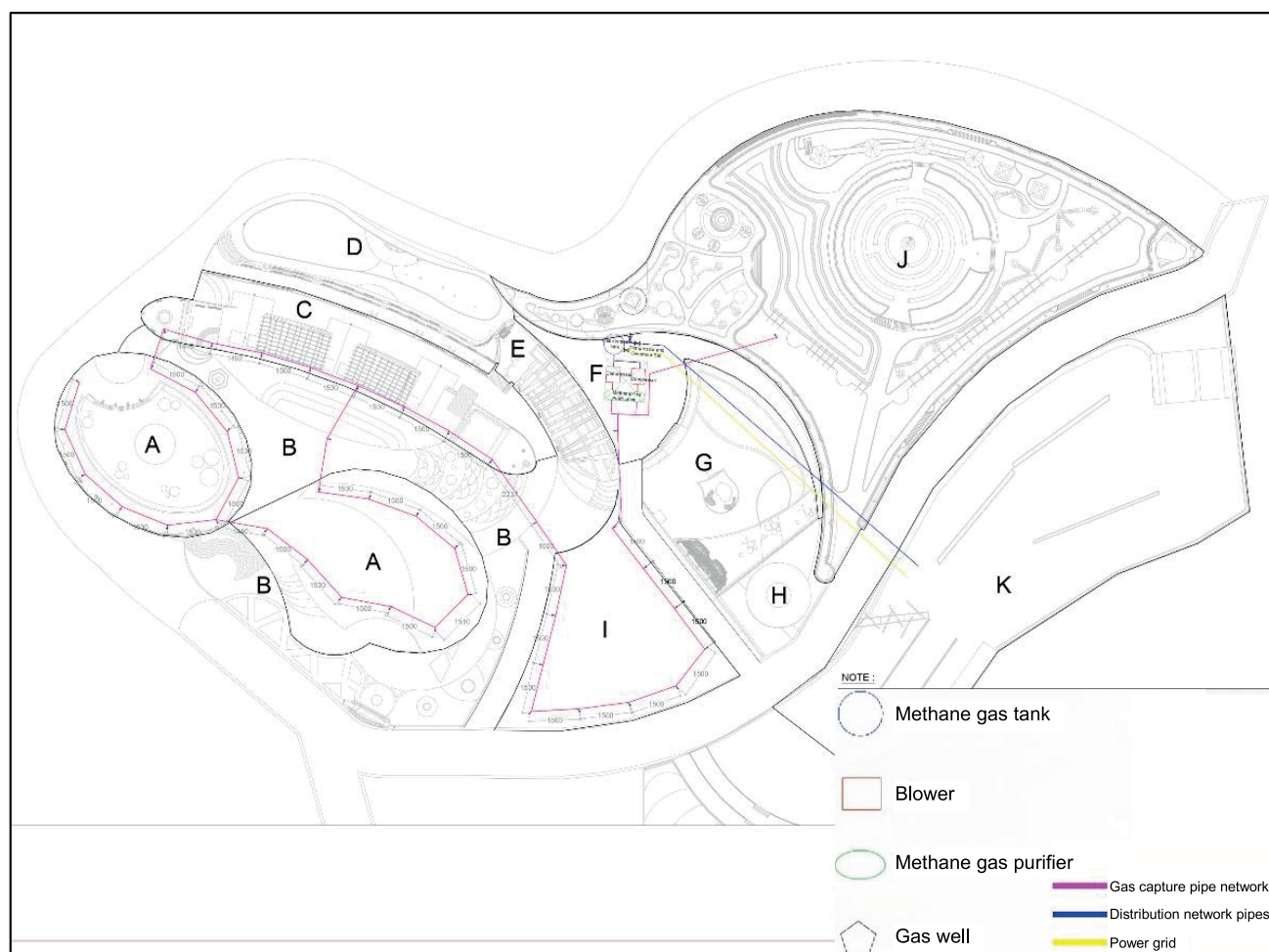
Fig. 2. Well location plan; A, B, C, D, E, F, G, H, I, J, K as in Tab. 2; source: own study
