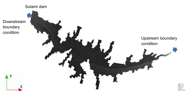
Fig. 3. Conceptual setup of the two-dimensional hydrodynamic-sediment transport solver in iRIC (Nays2DH) model for Sutami Reservoir; source: own study
