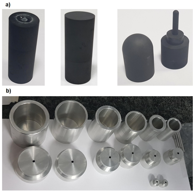
Fig. 1. Examples of reference workpieces of ionization chambers: a) graphite, b) PA6 aluminium alloy.
