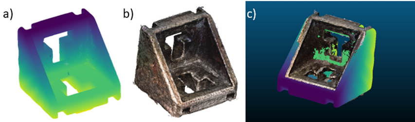
Fig. 2. Point cloud comparison: a) scanner reference, b) NeRF reconstruction of the metal bracket (coloured), c) aligned overlay.
