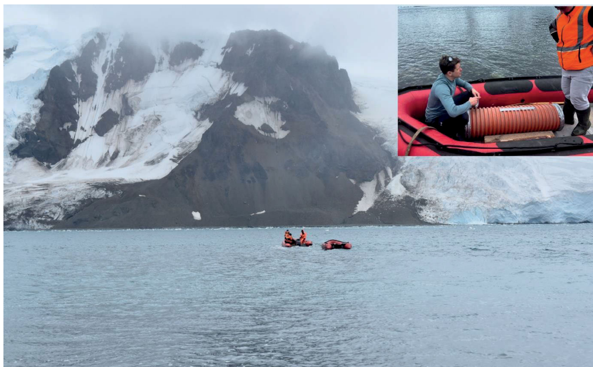
Fig. 3. Magnetometer setup for boat borne magnetic measurements in the Ezcurra Inlet.
