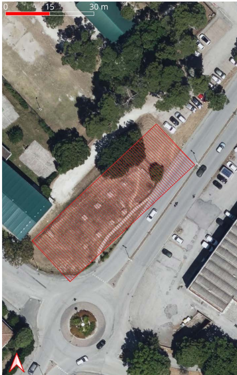
Fig. 5. The area covered by GPR surveys with the use of a 450 MHz antenna (photo and drawing: F. Welc).
